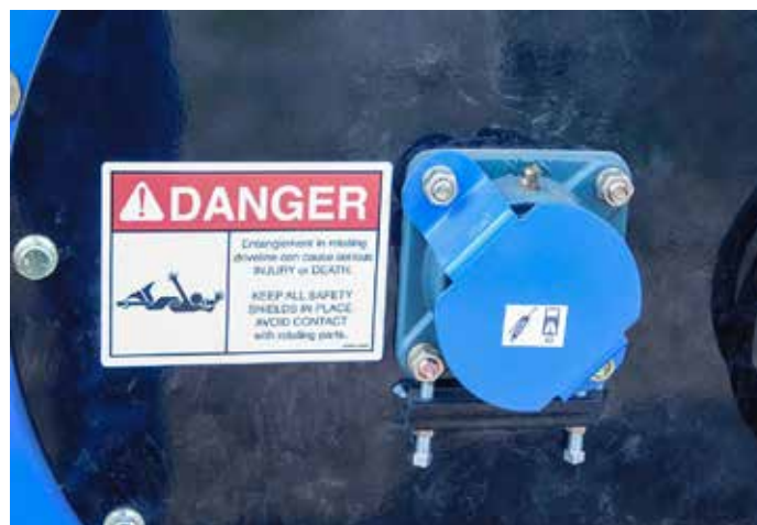
4. DANGER: Rotating Shaft Hazard
