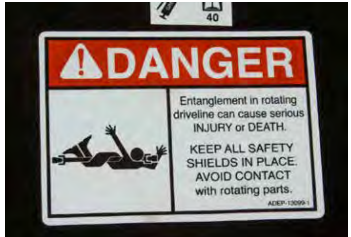
32. DANGER: Entanglement in rotating driveline
